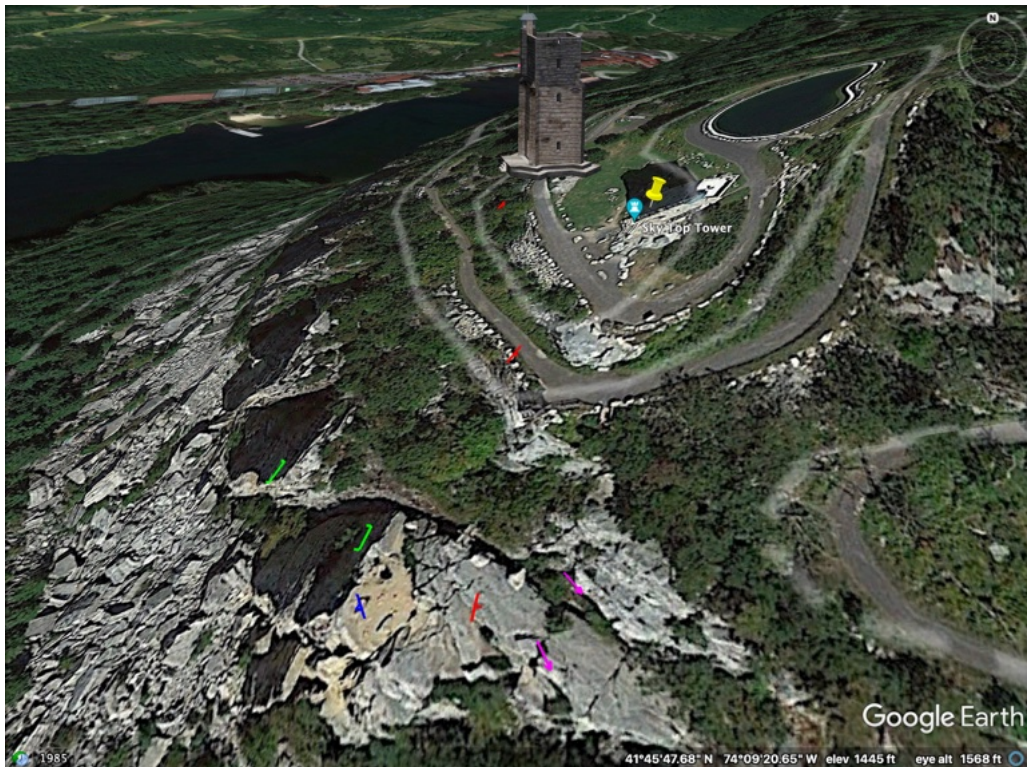
Figure 15.4: Example data (simulated) from the file Sky Top viewed in Google Earth. Example data types are S0 (bedding, red), S1 (cleavage, blue), J (joints, green), and a lineation (L, magenta).
