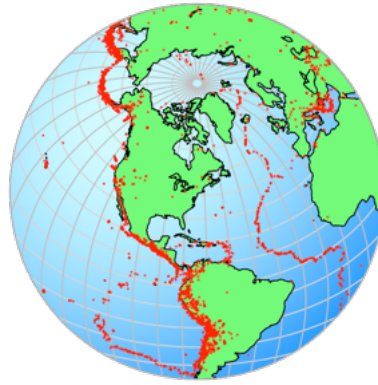
Figure 5.6: Upper hemisphere equal-area projections of 14,229 earthquake epicenters with magnitudes greater than 4.5 from 1980 to 1990 centered at latitude, longitude 41.764^\circ, -74.156^\circ by rotating the projection 74.156^\circ about the Z = \text{Top} axis, and then 41.764^\circ about the Y = \text{Right} axis. Data from NOAA.
